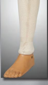
3D-Lite is an open weave polyester material, impregnated with a non-toxic resin. This unique combination results in a lightweight and breathable material that is ideal for fabrication.
