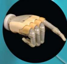
Index Point - facilitates operation of security key pads, ATM cash machines, cell phones key pads, touch screen registers, etc.
