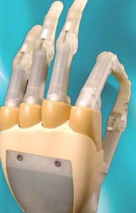
i-LIMB thumb can rotate through various grip positions in similar manner to the human thumb.
